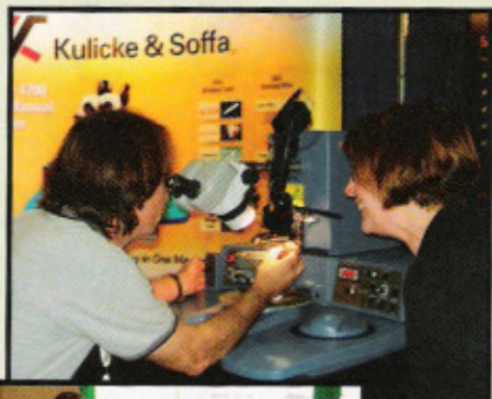
Joe Martin, manual wire bonder product marketing manager, Kulicke & Soffa, demonstrates the 4700 Convertible Wire Bonder. This manual benchtop bonding tool provides both wedge-wedge and ball-wedge bonding capabilities. It suits R&D environments, rework, and low-volume production.
