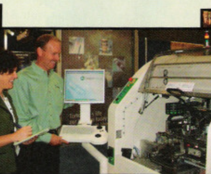
Gregg Taran, director, North America, Datacon, showed me the EVOO 2000 Die Bonder, which features a separate dispensing area with integrated dispenser and a bonding area for die-attach and flip chip applications. Datacon will be celebrating their 20 th anniversary in early December.
